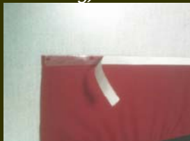
Pre-attach Glue Tape (For Sewfree heat Pressing)
