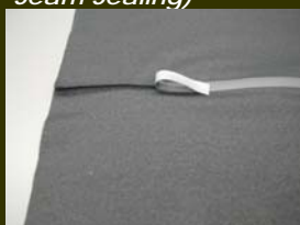
Line Bonding (work with Reinforcement Seam Sealing)
