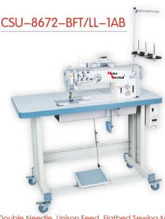
Double Needle, Unison Feed, Flatbed Sewing Machine. (Automatic Undertrimming & Backtacking, Pneumatic Presser Foot Lifting.) (Extra Large Hook) (For Heavy Materials)
