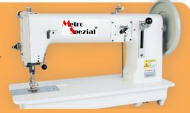
S.P.M. Model No. CS-243 800 Max. Stitch Lift Of Presser Foot Length (Knee) 15mm 20mm Needle System Needle Bar DY×3 #26 56mm  $(#23 \sim #28)$
