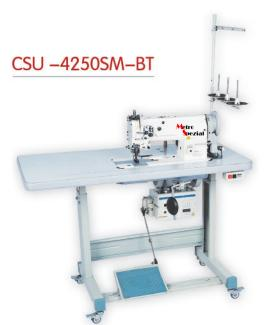
Double Needle, Flatbed Sewing Machine, With Unison Feed.(With automatic undertrimming & backtacking, smocking mechanism)(Large hook, for heavy materials)
