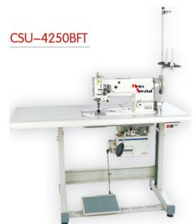
Double Needle, Flatbed Sewing Machine, With Unison Feed.(With automatic undertrimming & backtacking & presser foot lifting)(Large hook, for heavy materials)
