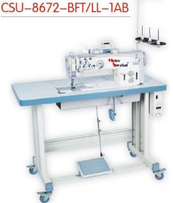
Double Needle, Unison Feed, Flatbed Sewing Machine. (Automatic Undertrimming & Backtacking, Pneumatic Presser Foot Lifting.) (Extra Large Hook) (For Heavy Materials)
