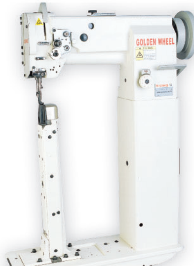
Single Needle, High-Postbed Sewing Machine, With Unison Feed. (Right-side postbed, Large hook)
