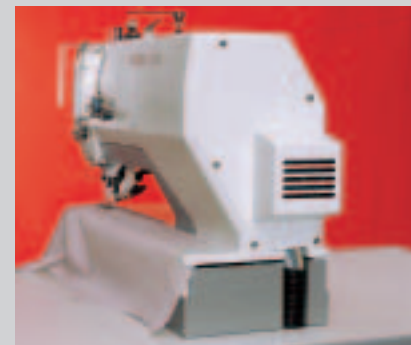
Servo sewing drive integrated in housing
