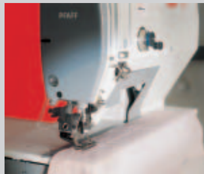
Off-set arm for easy placing/handling of workpiece
