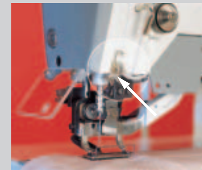
Thread monitor with optical sensor
